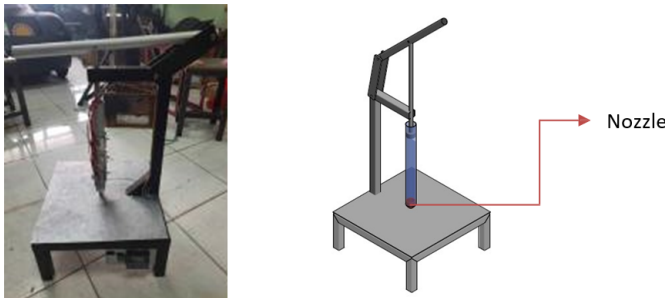
Fig. 1: Vertical Polymer Injection Molding.
