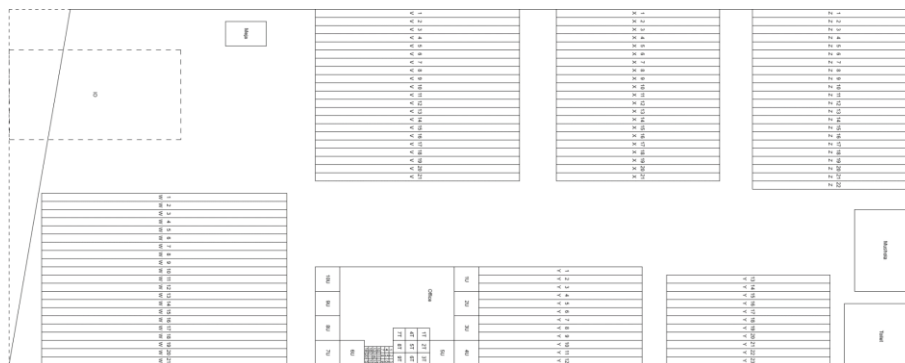
Figure 5. Proposed Layout Using Class-based and Dedicated Storage with Classification Based on Type and Size
