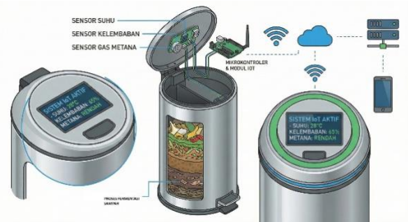
Fig. 2. The Design of IoT-based composter monitoring system
