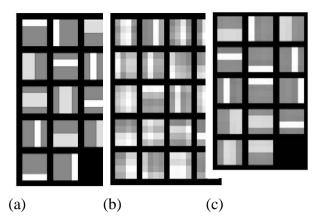
**Figure II.1** Extended bar problem solution obtained from PE-NMF: (a) source images, (b) mixed images, (c) recovered images from PE-NMF. (Zhang et all, 2008)
